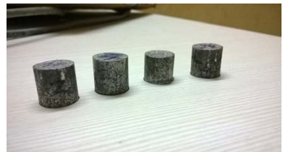
Figure 2 Al-6082 Sic Samples of Different Compositions used for Wear test
