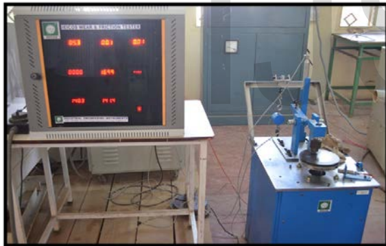
Figure 3 Pin-On-Disc Friction and Wear tester
